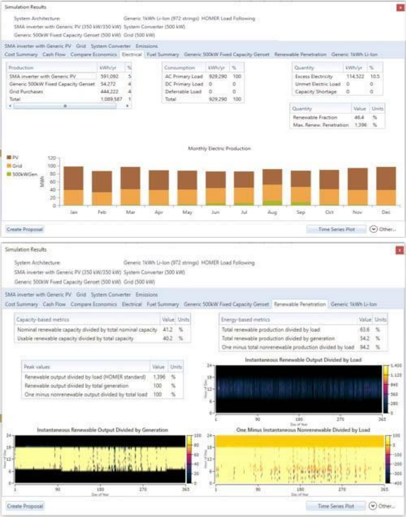
The graphs show HOMER Pro's comparison of production from different energy resources and varying electrical consumption, as well as the total load met by renewable energy.
