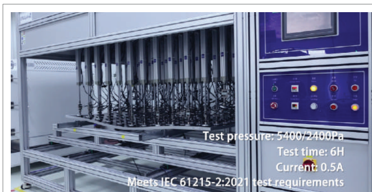
Figure (3): Applying 5400 Pa & 2400 Pa Positive and Negative Pressure to Frontsheet and Backsheet of Panels while Conducting Static Mechanical Load Test
